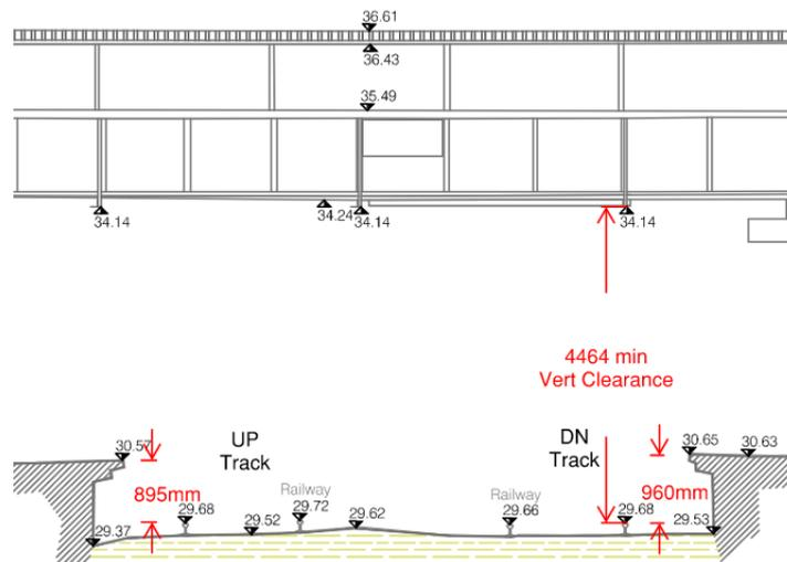
Figure 4: Clearances beneath OBB 81 (northern elevation)
