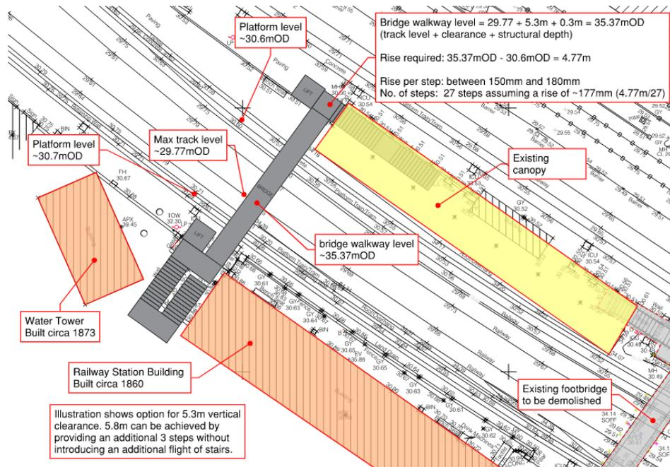
Figure 11: Plan view showing new bridge option north of existing crossing
