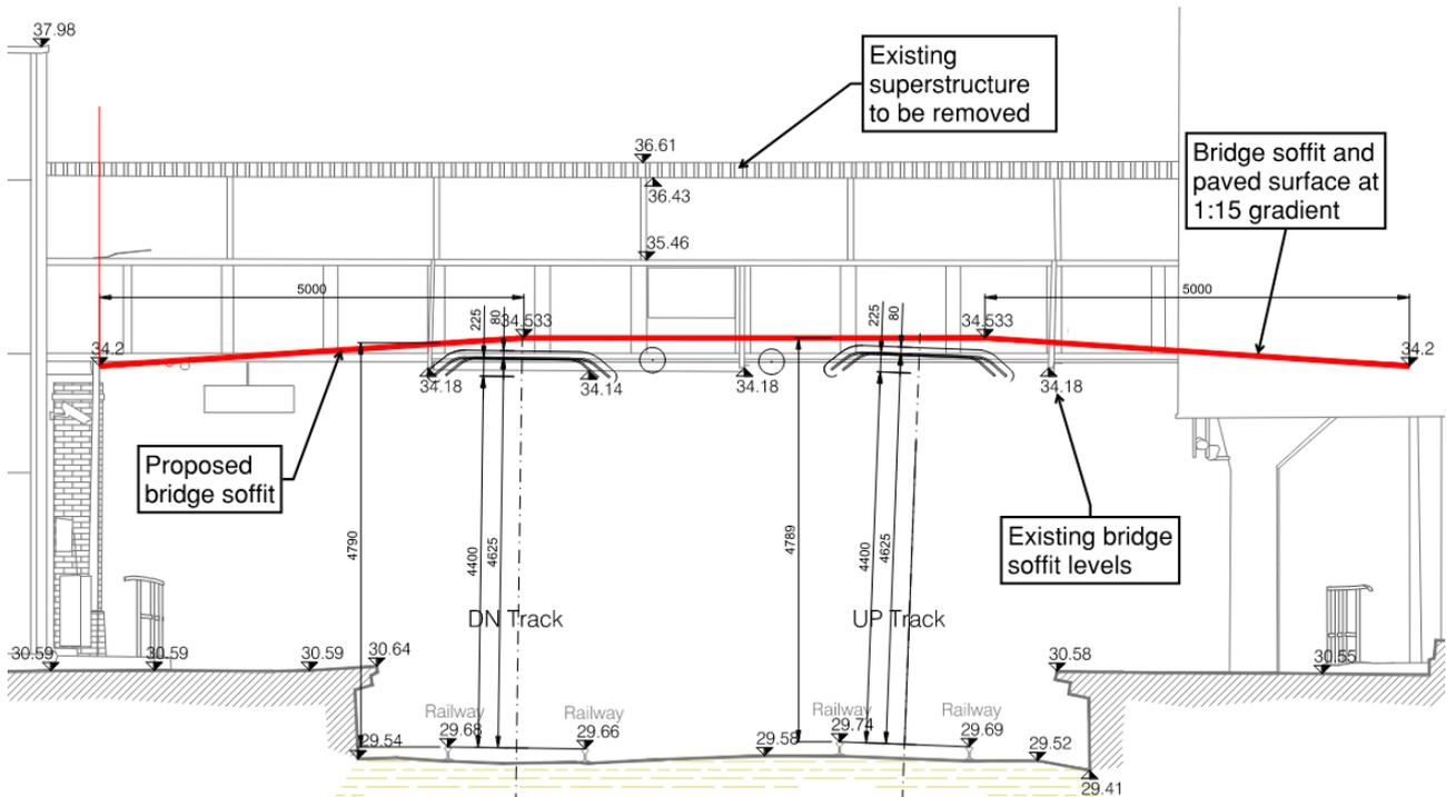
**Figure 10: Elevation of proposed superstructure replacement at OBB81**
