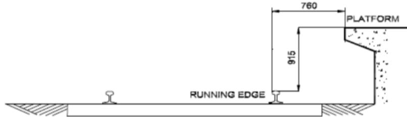
**Figure 5: Required platform clearance (extract from I-PWY-1101- Figure 2.1)**
