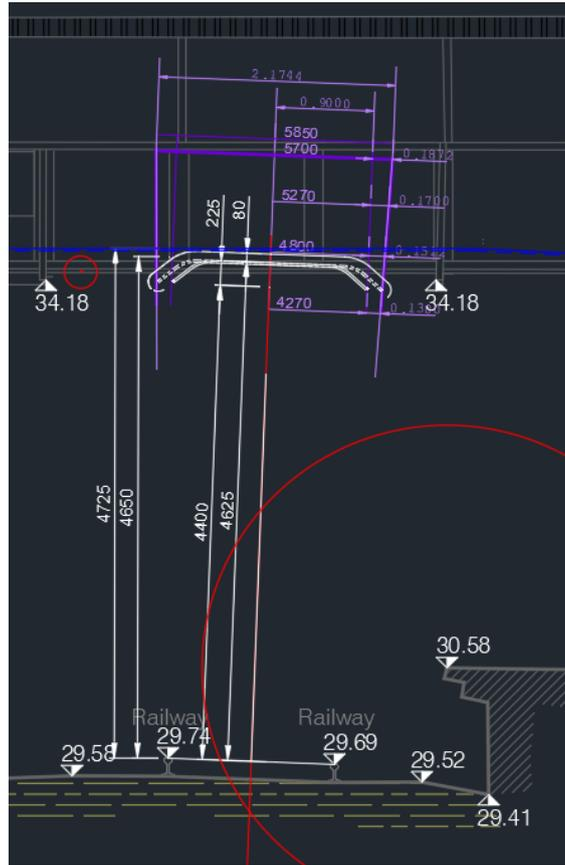
Figure 9: Pantograph envelope utilising a CWH of 4.400 m (UP-track looking north)
